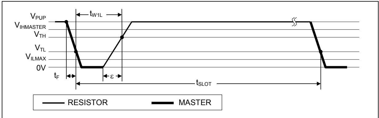
Figure 13. READ/WRITE TIMING DIAGRAM
