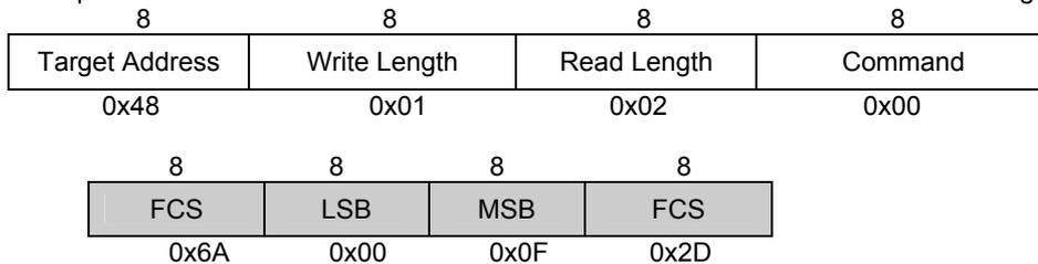
**Figure 8. Get Internal Temperature Command Example**
