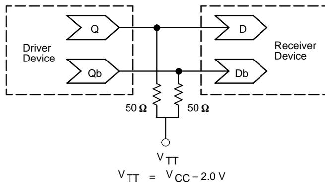
**Figure 1. Typical Termination for Output Driver and Device Evaluation**
