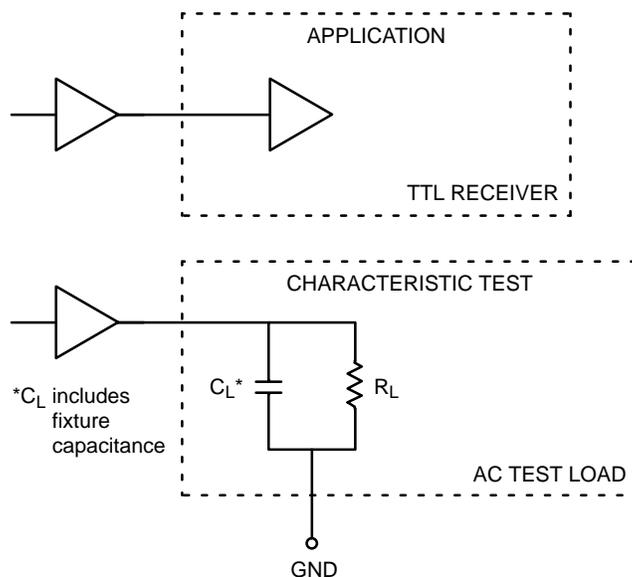
Figure 2. TTL Output Loading Used for Device Evaluation
