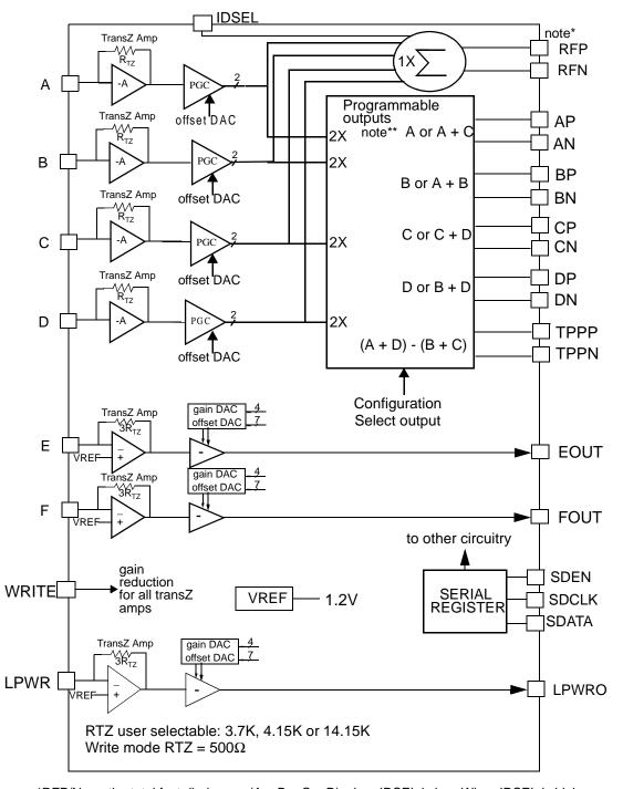
\*RFP/N are the total fast diode sum (A + B + C + D) when IDSEL is low. When IDSEL is high RFP/N output is right channel minus the left channel (A+D) - (B+C).
