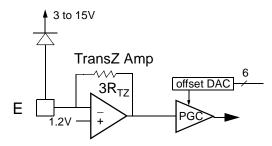
Each amplifier also has a dedicated 6-bit offset DAC controllable though the serial register. Input/Output bias level for zero input current is set at 1.2V. Tables for TZ gain and PGC are given below.
