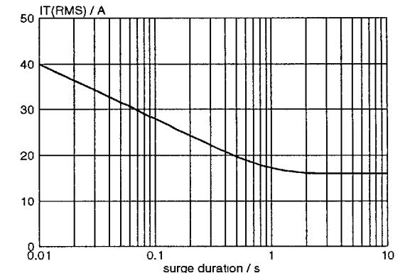
Fig.5. Maximum permissible repetitive rms on-state current  $I_{T(RMS)}$ , versus surge duration, for sinusoidal currents,  $f = 50\text{ Hz}$ ;  $Ths \leq 38^\circ\text{C}$ .
