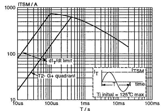
Fig.2. Maximum permissible non-repetitive peak on-state current  $I_{TS(M)}$ , versus pulse width  $t_p$ , for sinusoidal currents,  $t_p \leq 20\text{ms}$ .
