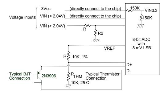
Figure 1. Hardware monitor configuration
