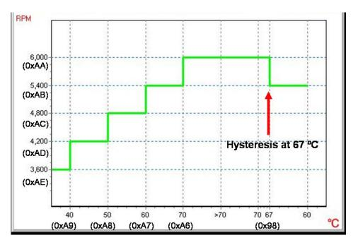
Figure 9 Stage mode fan control illustration-3
