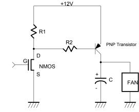
Figure 6 +12/5V PWM fan control application circuit
