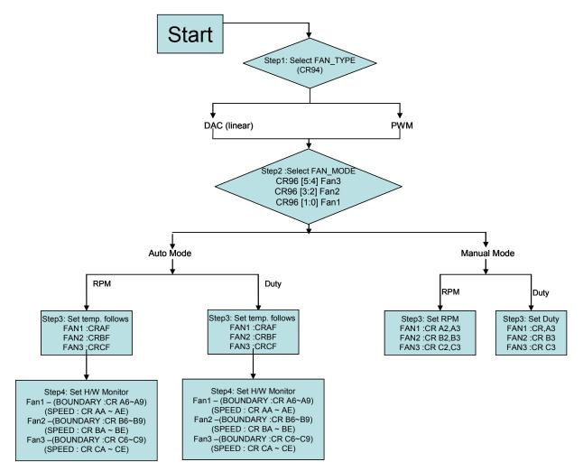
Figure 7 Fan type & mode selection flow
