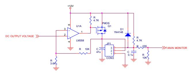
Figure 5 DAC fan control application circuit
