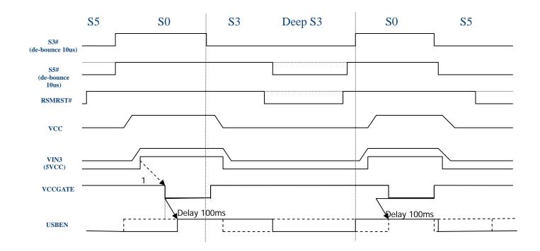
Figure 24 VCCGATE & USBEN timing
