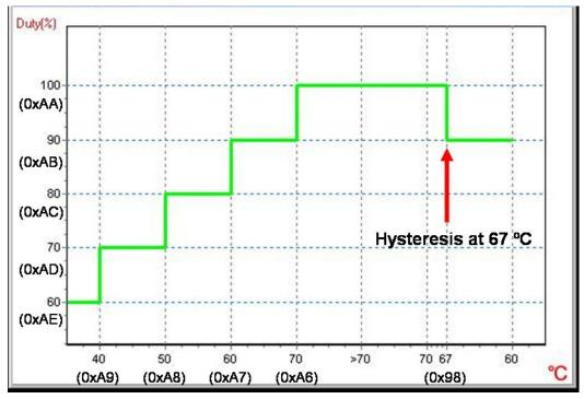
Figure 8 Stage mode fan control illustration-2
