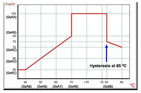
Figure 10 Linear mode fan control illustration-1
