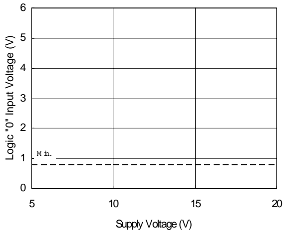
Figure 9B. Logic "0" Input Voltage vs. Supply Voltage
