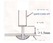
(2)當用手工來彎曲引線時,請遵照下列方法When the lead needs to be bent by hand, please follow the instruction as below: 用手指捏住圓柱晶體的外殼;用鑷子夾住引線要彎曲的部位,該部位離晶體基座底部1.5mm以上(推薦3.0mm);用鑷子夾住彎曲引線成90°,不要用力拉引線。用力拉引線可能造成引線根部的玻璃子破裂,而產生漏氣損壞元件電性能。Hold the body of the cylinder type crystal unit in fingers;
