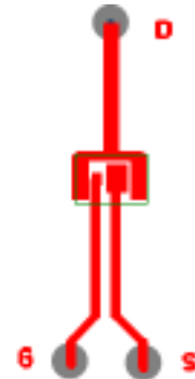
⑩ Mounted on minimum footprint full size board with metalized back and with small clip heatsink (still air)
