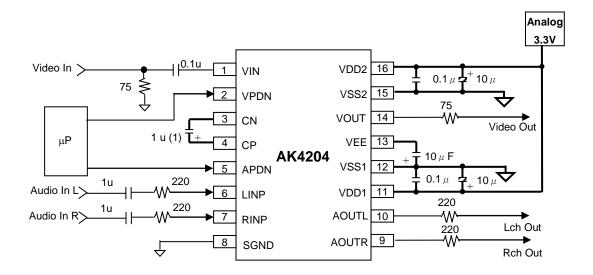
Figure 8. Typical Connection Diagram
