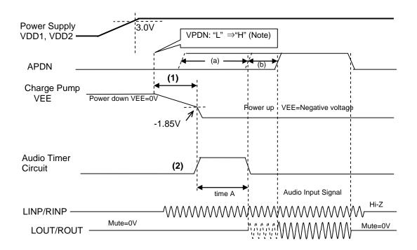
Figure 6. System Reset Diagram
