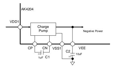
Figure 3. Charge Pump Circuit
