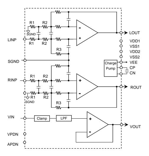
Figure 1. AK4204 Block Diagram
