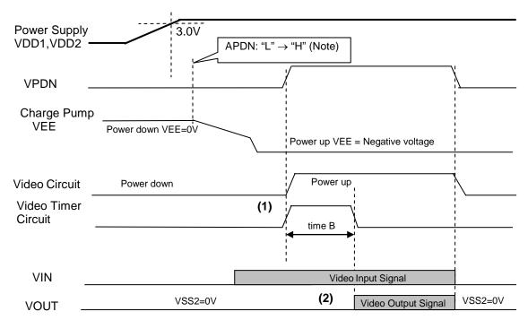
Figure 7. System Reset Diagram
