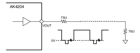
Figure 5. Video Signal Output
