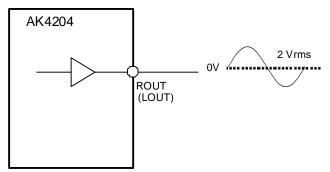
Figure 4. Audio Signal Output
