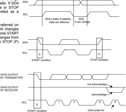
Legend \_\_\_\_\_\_\_ The mastering side is a transmitter. A Acknowledge S Start condition Sr Repetition start condition The slave side is a receiver. A Unacknowledged P Stop condition
