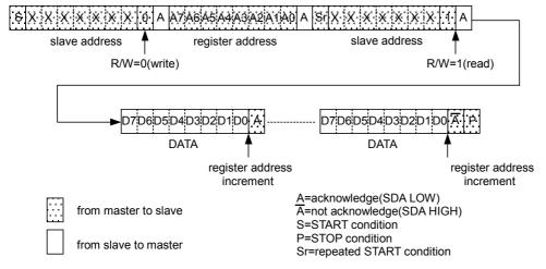
X As for reading protocol and multiple reading protocols, please do A(not acknowledge) after doing the final reading operation. It stops with read when ending by A (acknowledge), and SDA stops in the state of Low when the reading data of that time is 0. However, this state returns usually when SCL is moved, data is read, and A (not acknowledge) is done.
