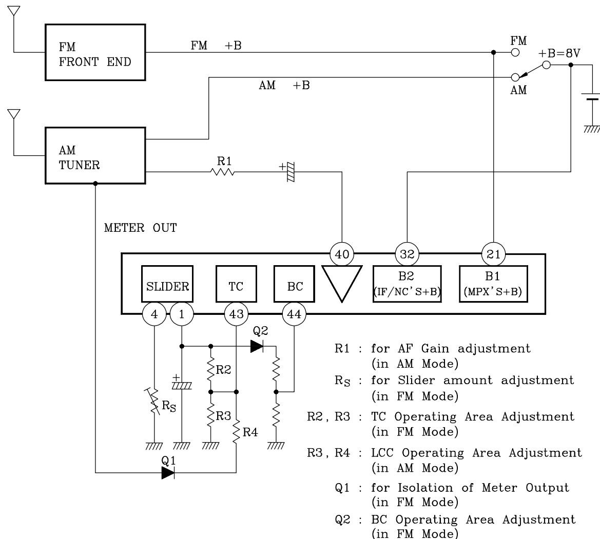
In case of B1="L" level in AM mode, use Slider input terminal (pin 10) which AM tuner output signal goes to the slider circuit (but, In case of FM mode, this pin is for meter output).
