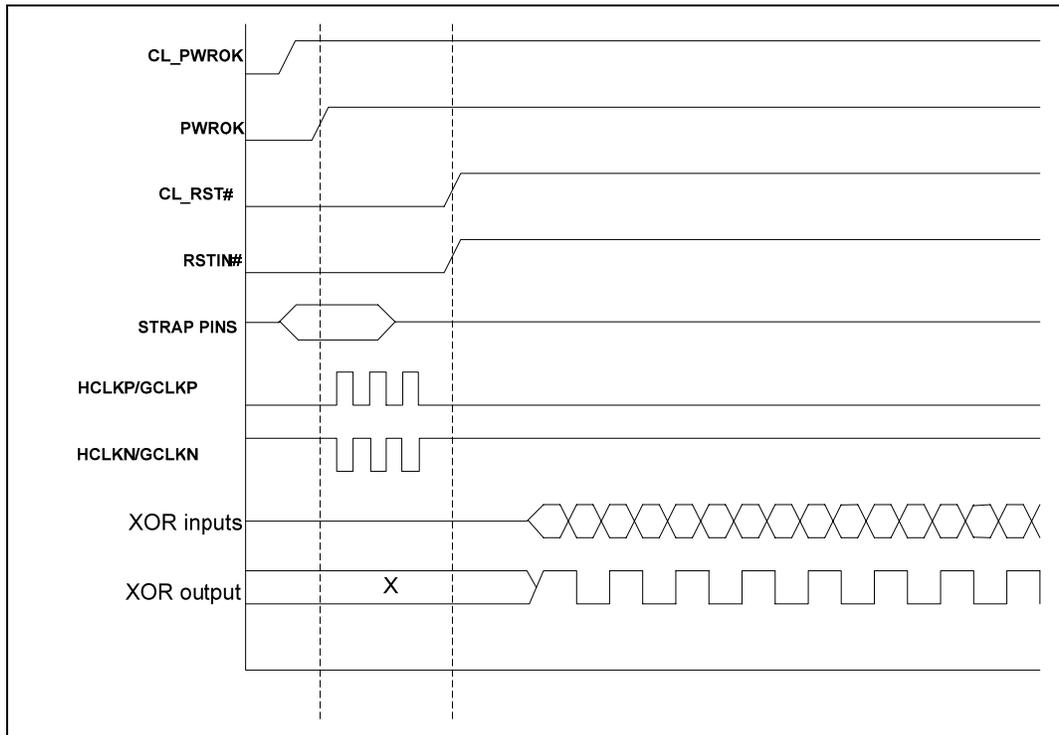
The above figure shows the wave forms to be able to boot the part into XOR mode. The straps that need to be controlled during this boot process are BSEL[2:0], SDVO\_CTRLDATA, EXP\_EM, EXP\_SLR, and XORTEST.
