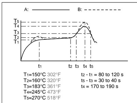
Temperature rise of relay itself may vary according to the mounting level or the heating method of reflow equipment.
