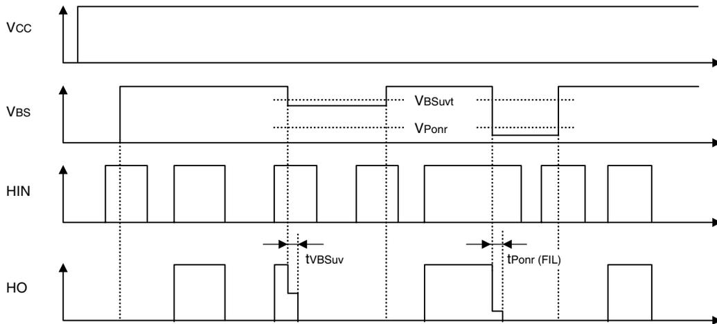
\* When supply voltage is lower than Vponr, then output will go low after tPonr(FIL).
