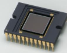
S9978 is FFT-CCD area image sensor specifically designed for low-light-level detection in scientific applications. S9978 also features low noise and low dark current (MPP mode operation). These enable low-light-level detection and long integration time, thus achieving a wide dynamic range.
