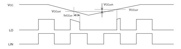
When Vcc Supply Voltage keeps lower UV Trip Voltage (VcCuvt = VcCuvr-VcCuvh) for Vcc Supply UV Filter Time, output signal becomes "L". And then, when Vcc Supply Voltage is higher than UV Reset Voltage, input signal (LIN) is L; output signal HO becomes "H".
