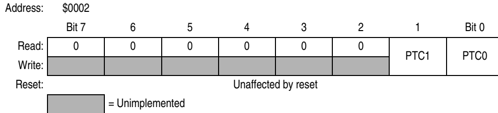
Figure 12-9. Port C Data Register (PTC)
