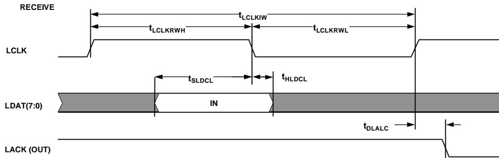
Figure 29. Link Ports—Receive
