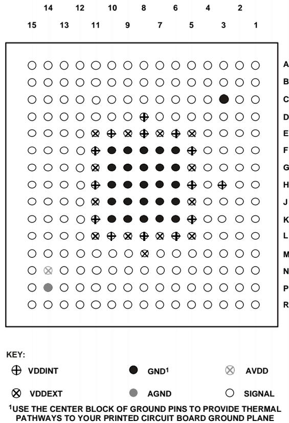
Figure 43. 225-Lead Metric MBGA Pin Assignments (Bottom View, Summary)
