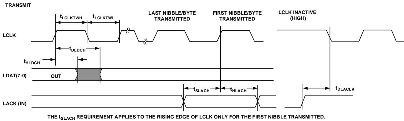
Figure 30. Link Ports—Transmit
