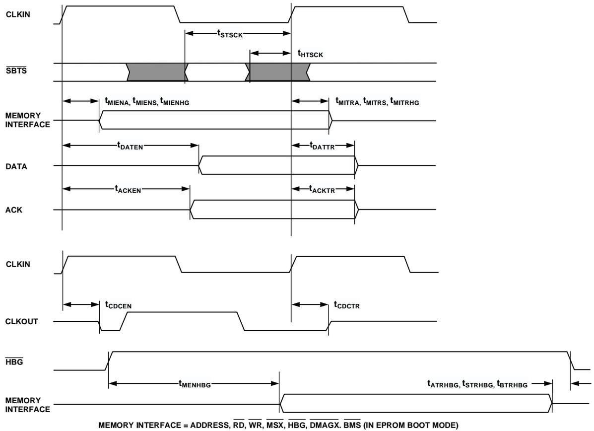
Figure 26. Three-State Timing
