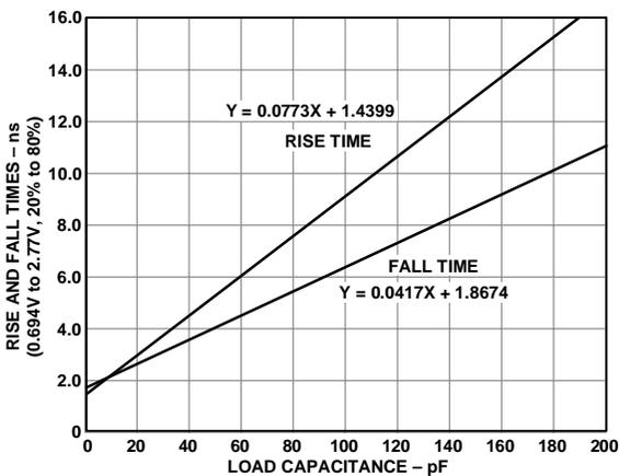
Figure 42. Typical Output Rise/Fall Time (20% - 80%,  $V_{DDEXT} = Min$ )
