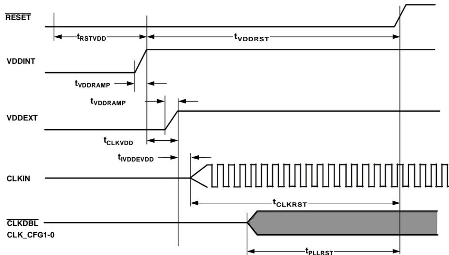
Figure 11. Power-Up Sequencing for Revisions 0.3, 1.0, and 1.1
