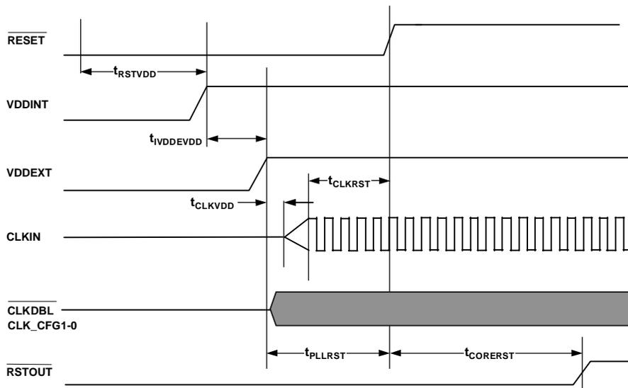
*Figure 12. Power-Up Sequencing for Revision 1.2*
