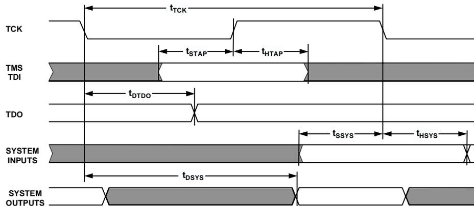
Figure 35. IEEE 11499.1 JTAG Test Access Port
