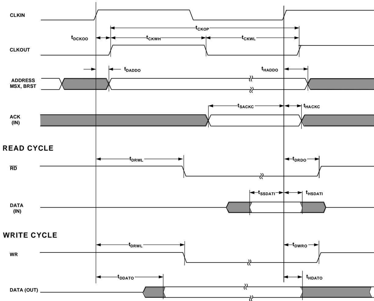
Figure 22. Synchronous Read/Write – Bus Master
