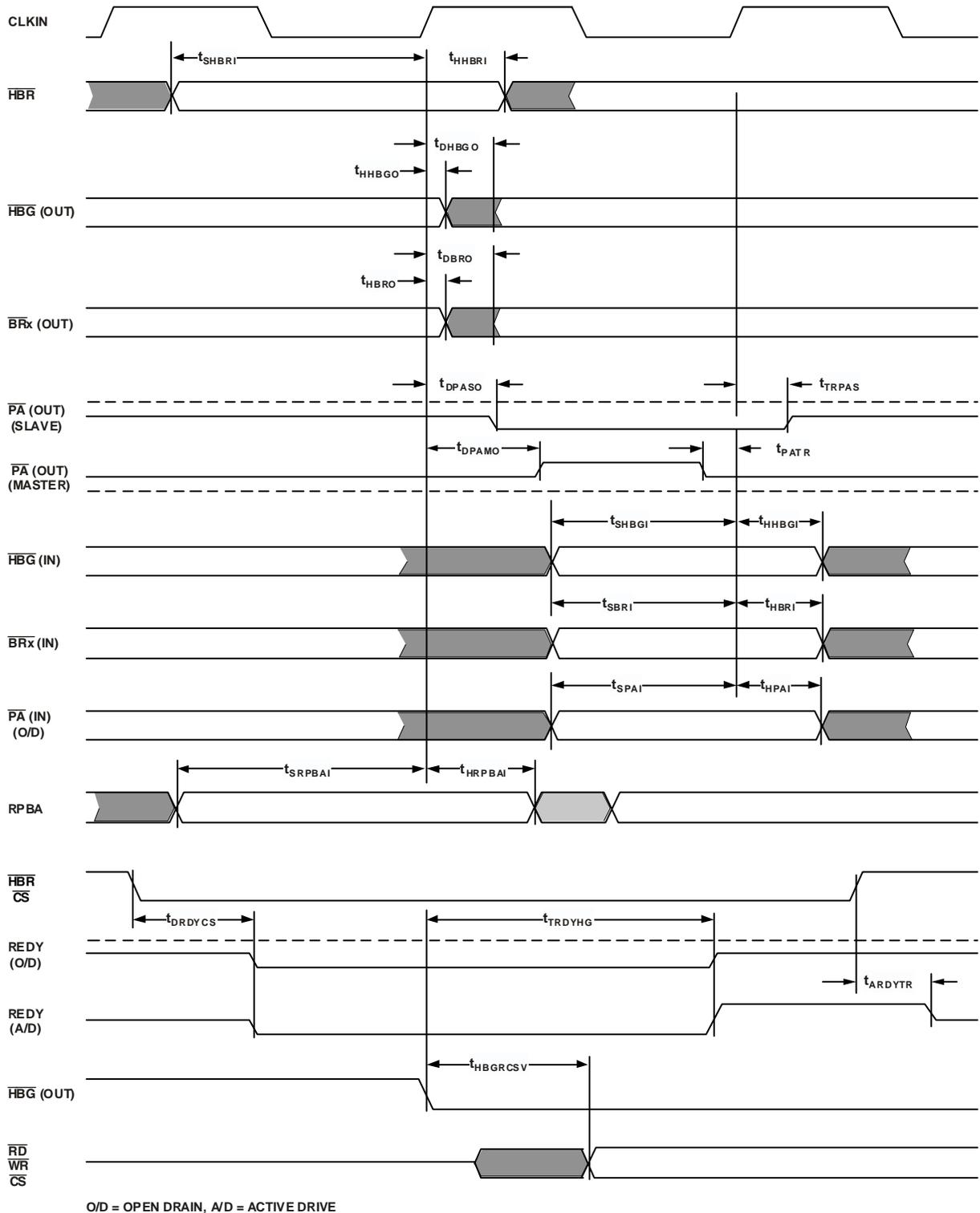
Figure 24. Multiprocessor Bus Request and Host Bus Request
