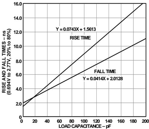
Figure 41. Typical Output Rise/Fall Time (20% - 80%,  $V_{DDEXT} = Max$ )
