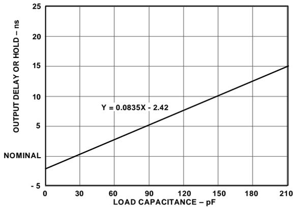
Figure 40. Typical Output Delay or Hold vs. Load Capacitance (at Max Case Temperature)
