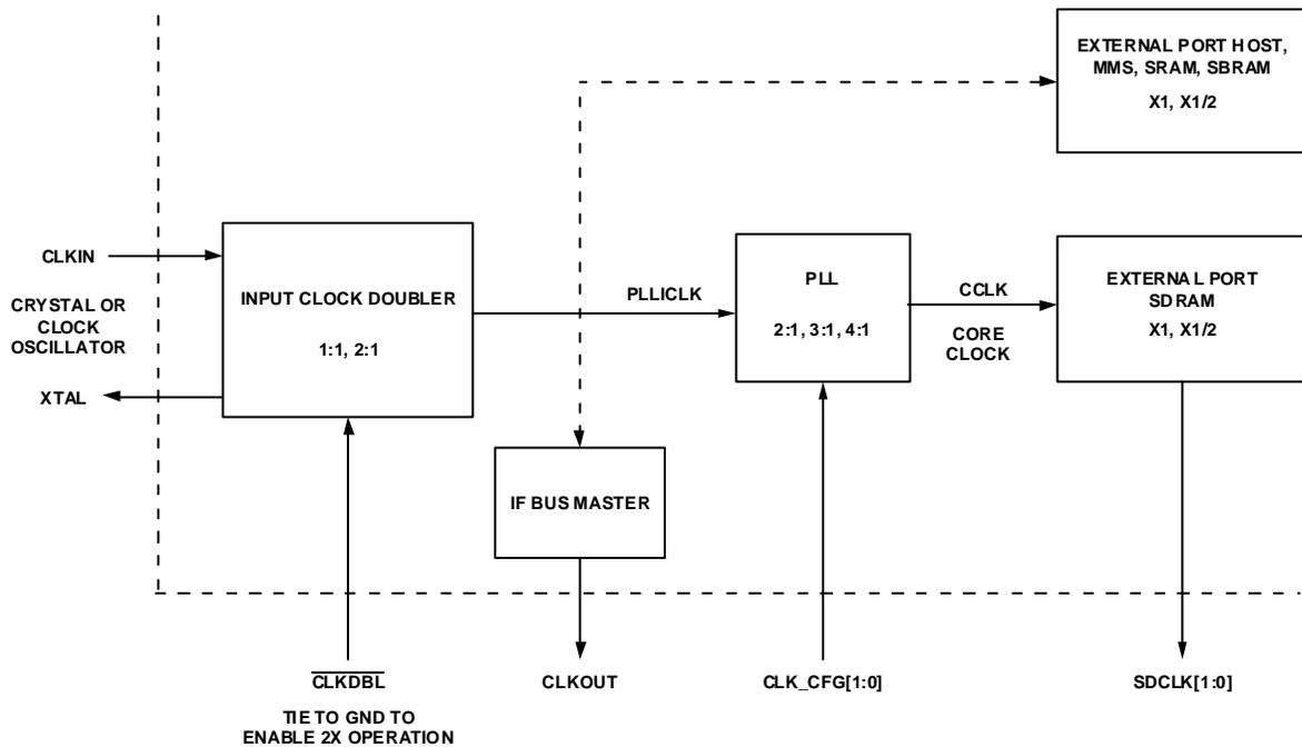
Figure 10. Core Clock and System Clock Relationship to CLKIN
