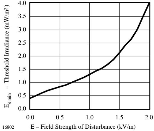
Figure 4. Threshold Irradiance vs. Field Strength of Disturbance
