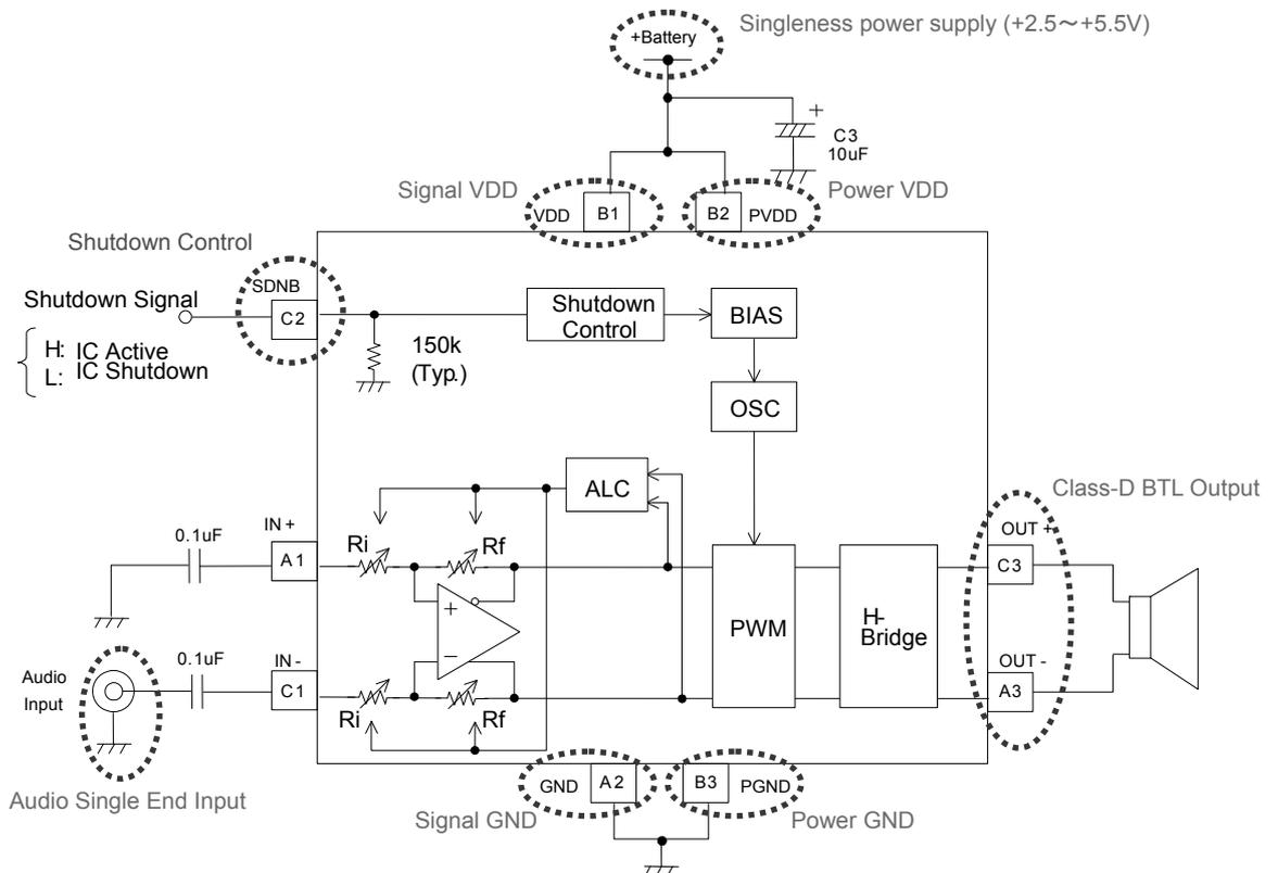
Fig4. Single end input (during IN- Input)
