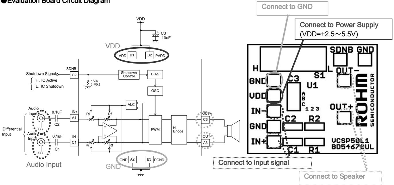
※Power Supply terminals VDD(B1), PVDD(B2) are SHORT in the board pattern and use a single power.
