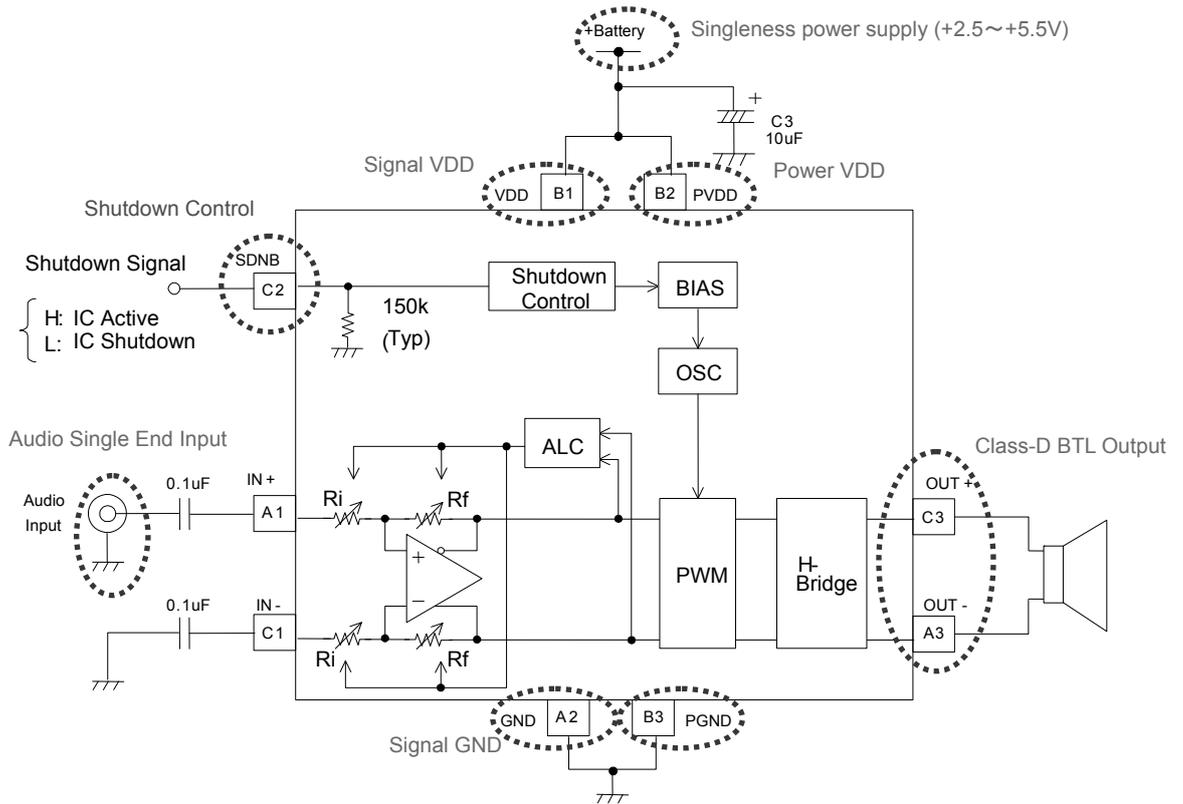
Fig3. Single end input (during IN+ input)
