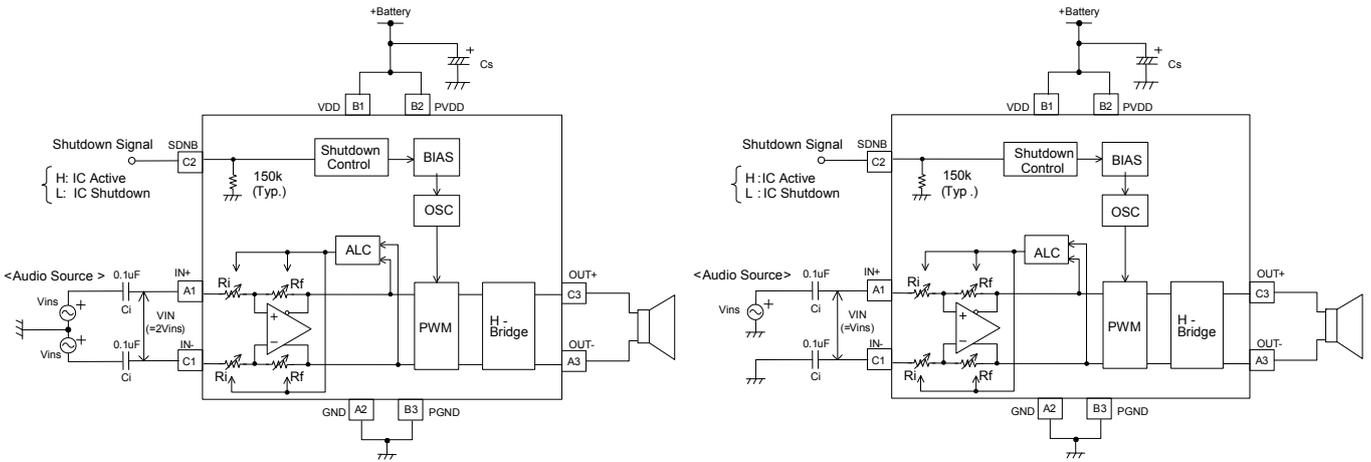
When Input Level is calculated at IC typical and audio source typical, when input coupling capacitor (Ci) value is large enough, every gain during the differential input and single end input will become:
