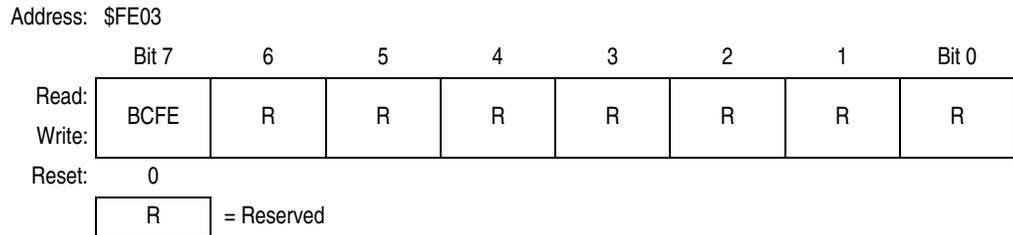
**Figure 14-20. SIM Break Flag Control Register (SBFCR)**
