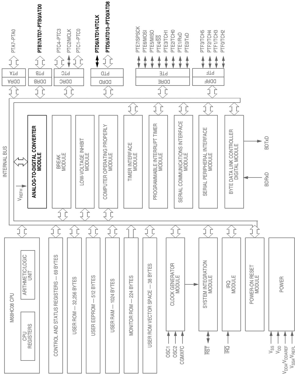
Figure 3-1. Block Diagram Highlighting ADC Block and Pins
