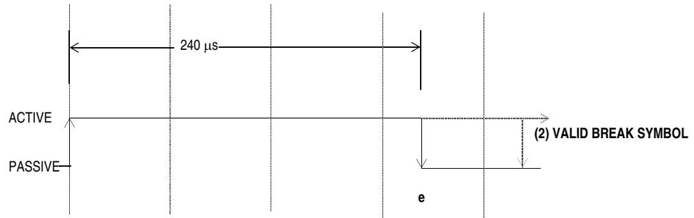
**Figure 4-12. J1850 VPW Received BREAK Symbol Times**
