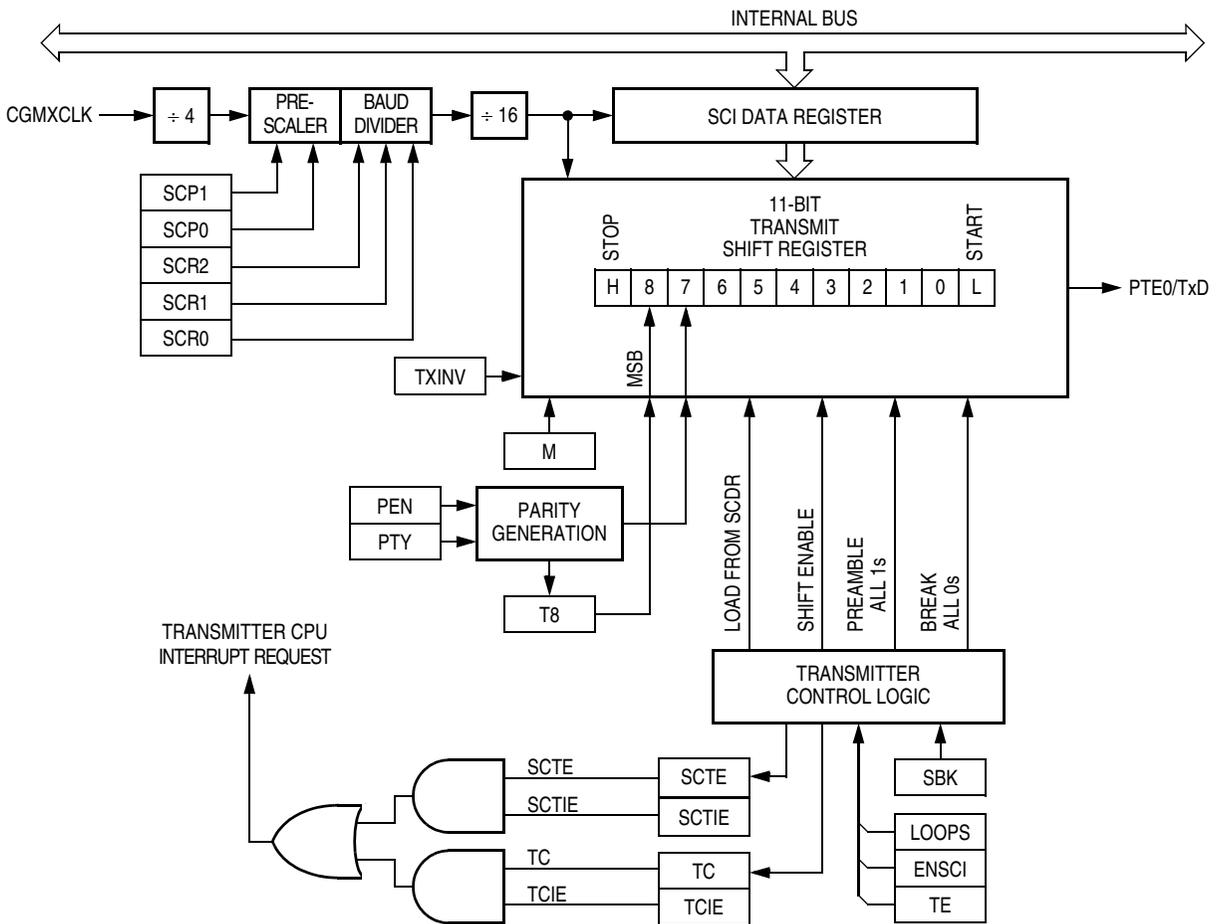
Figure 13-5. SCI Transmitter
