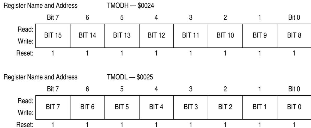
Figure 16-7. TIM Counter Modulo Registers (TMODH and TMODL)
