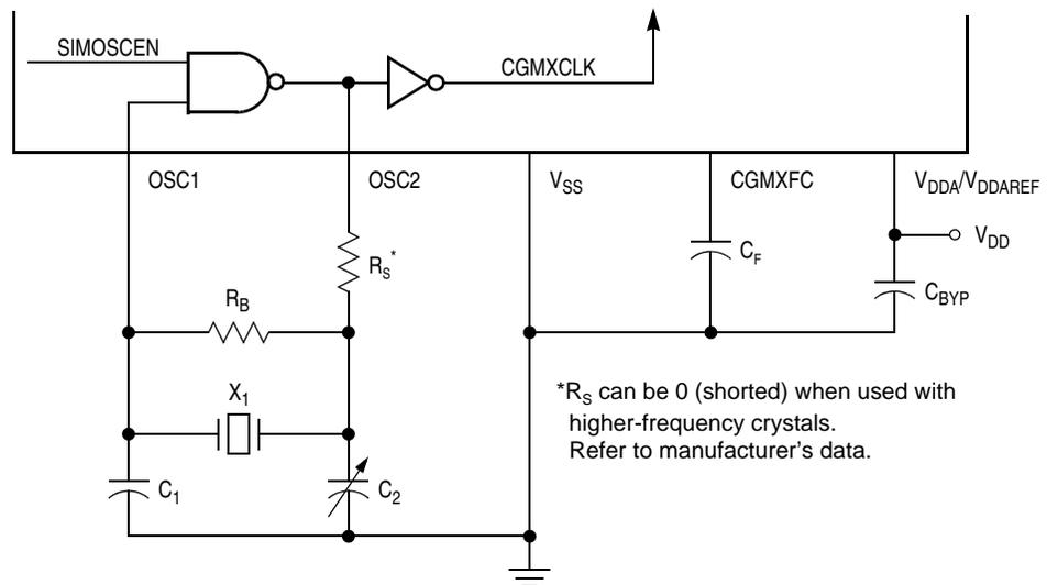
Figure 5-3. CGM External Connections
