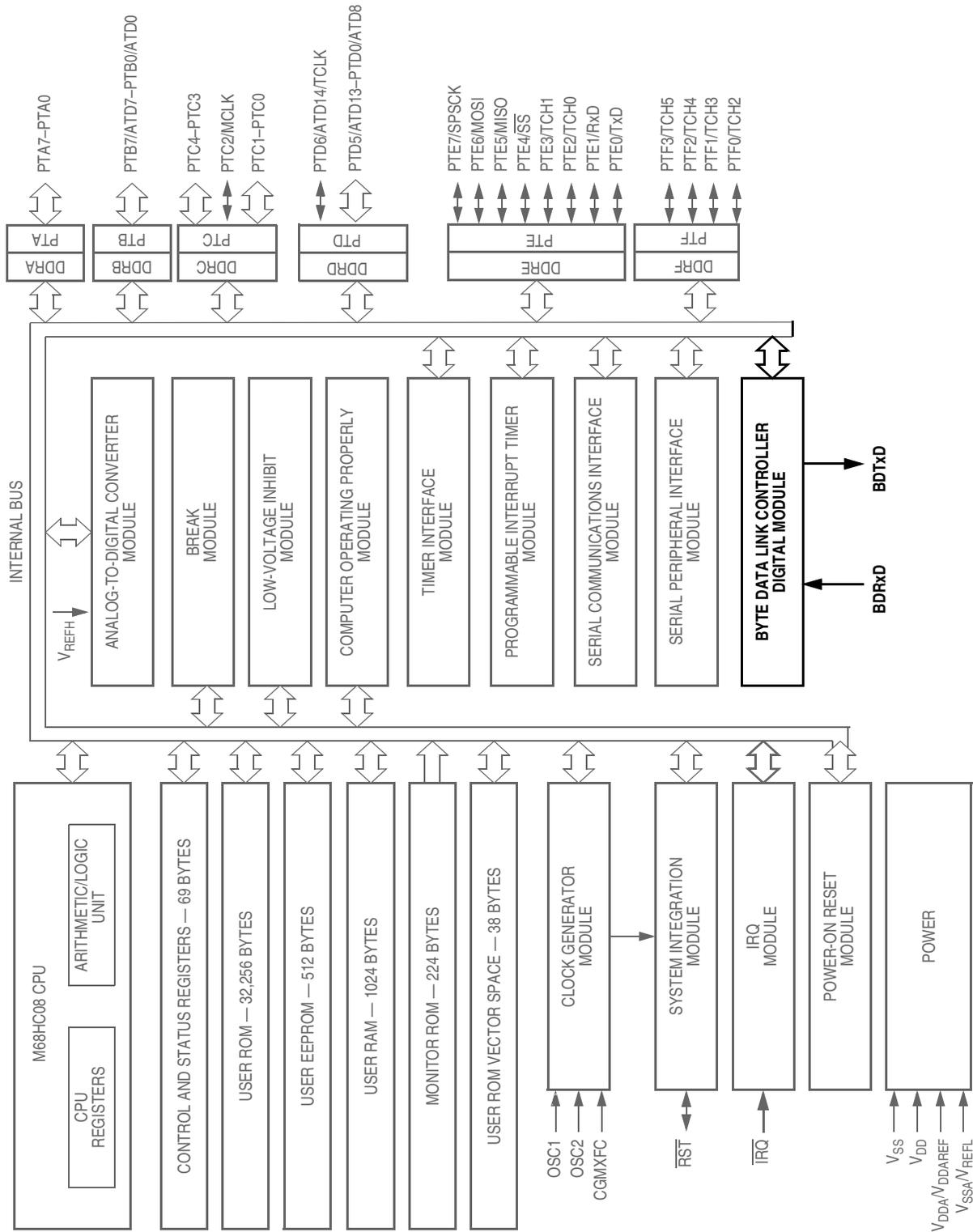
Figure 4-1. Block Diagram Highlighting BDLC Block and Pins
