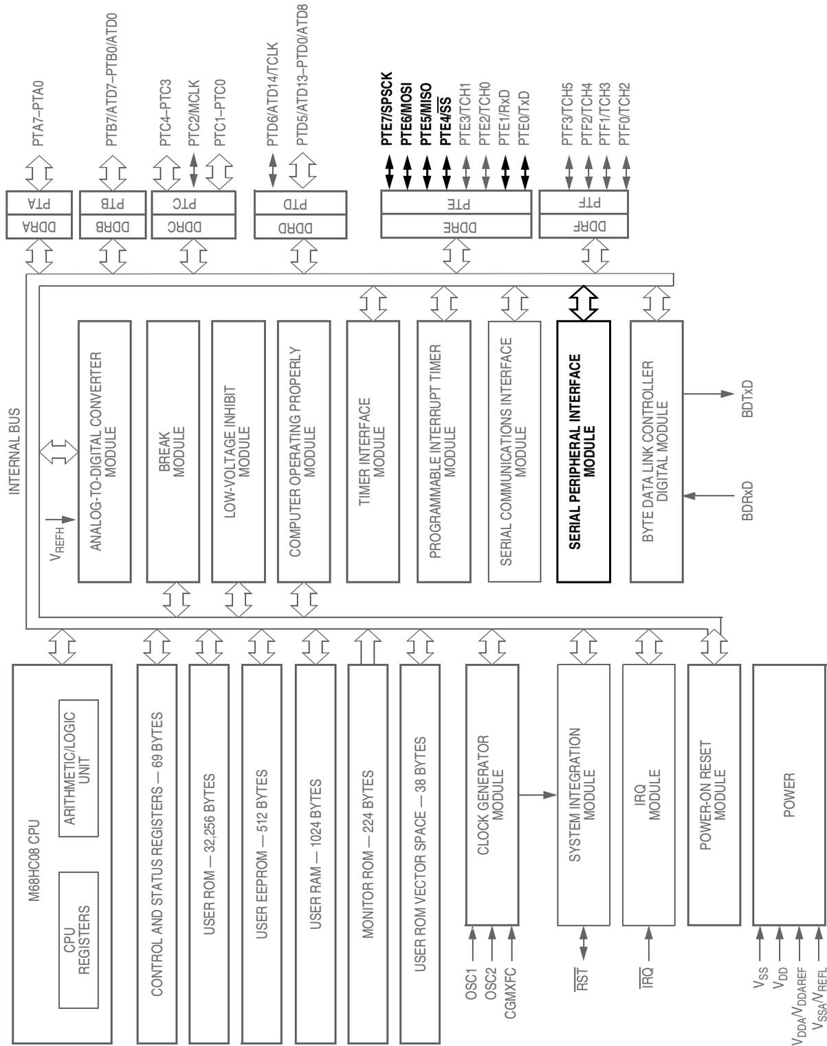
Figure 15-1. Block Diagram Highlighting SPI Block and Pins
