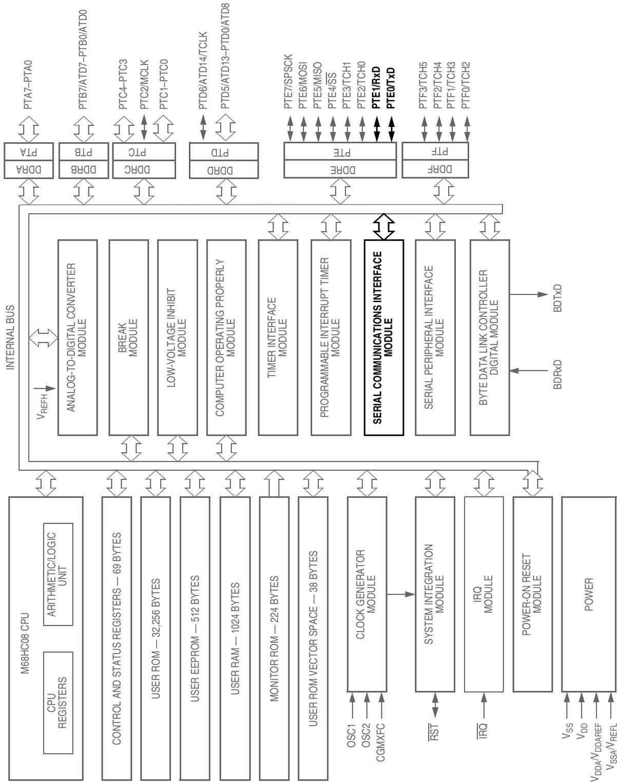
Figure 13-1. Block Diagram Highlighting SCI Block and Pins
