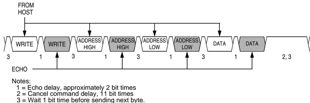
Figure 17-11. Write Transaction
