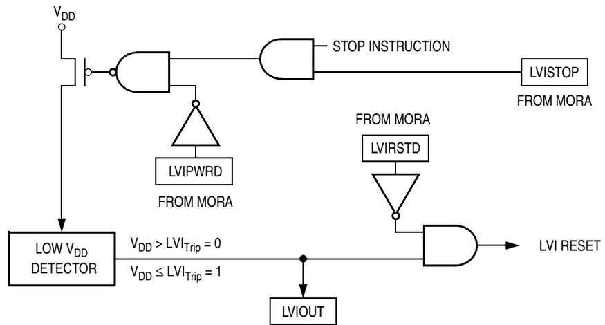
Figure 9-1. LVI Module Block Diagram
