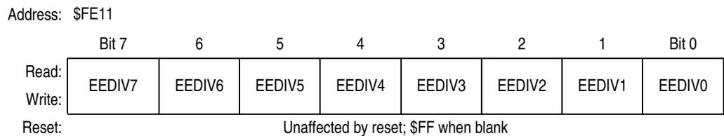
Figure 2-9. EEPROM Divider Non-Volatile Register Low (EEDIVLNVR)
