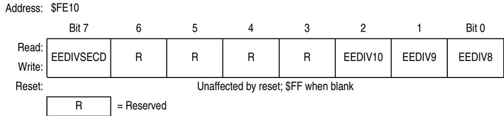
Figure 2-8. EEPROM Divider Non-Volatile Register High (EEDIVHNVR)
