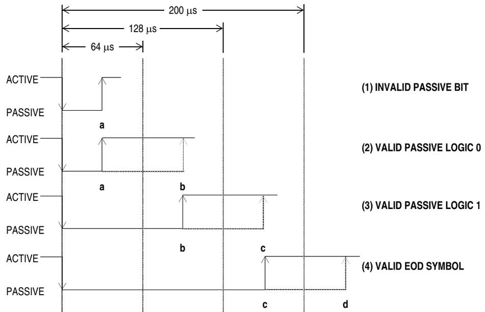
**Figure 4-9. J1850 VPW Received Passive Symbol Times**
