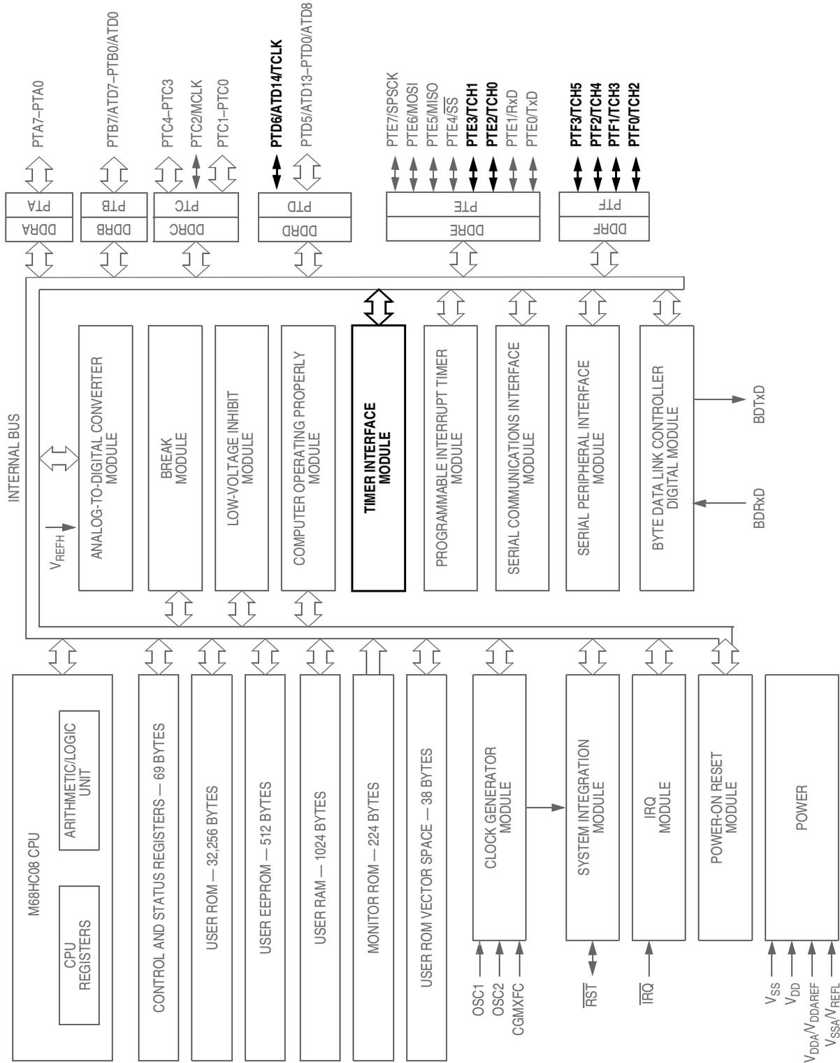
Figure 16-1. Block Diagram Highlighting TIM Block and Pins
