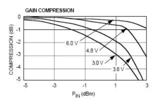
1. All data measured at TA = +25°C and VG1, VG2 adjusted for first stage quiescent current of 30 mA and second stage current of 65 mA, respectively.
