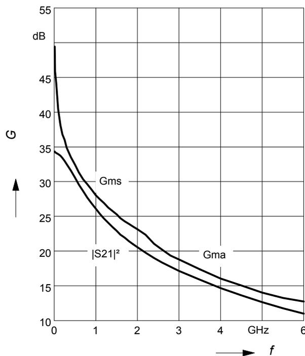
**Power gain  $G_{ma}$ ,  $G_{ms} = f(V_{CE})$**
