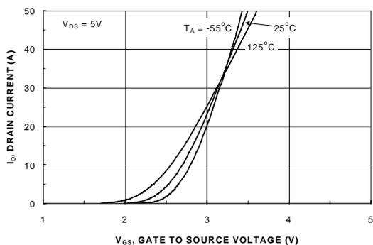
Figure 5. Transfer Characteristics
