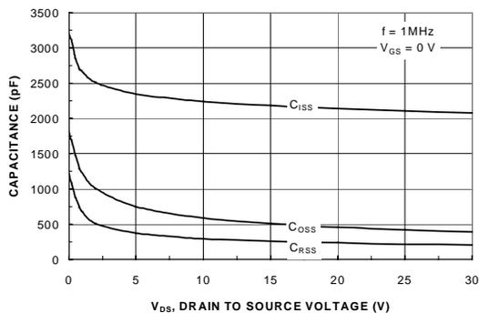
Figure 8. Capacitance Characteristics
