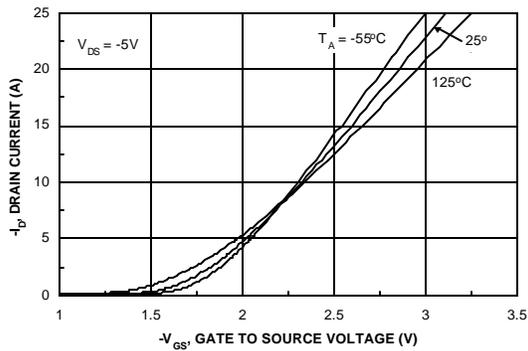
Figure 5. Transfer Characteristics.
