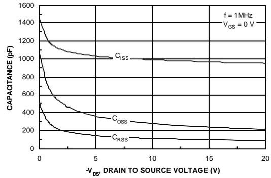
Figure 8. Capacitance Characteristics.
