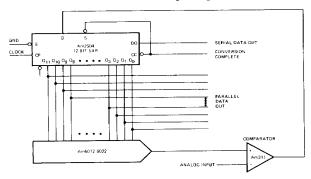
This shows how the Am2502/3/4 registers are used with a Digital-to-Analog converter and a comparator to form a very high-speed continuous conversion Analog-to-Digital converter. Conversion time is limited mainly by the speed of the D/A converter and comparator with typical conversion rates of 100,000 conversions per second.
