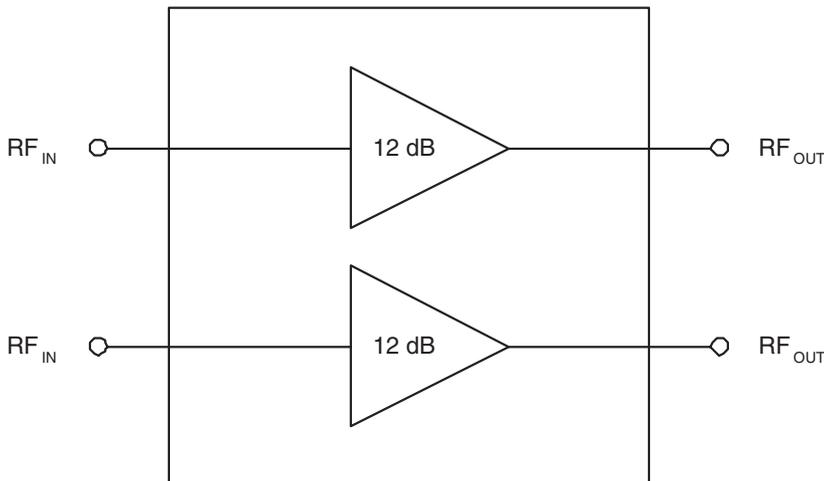
**Figure 1: Block Diagram**
