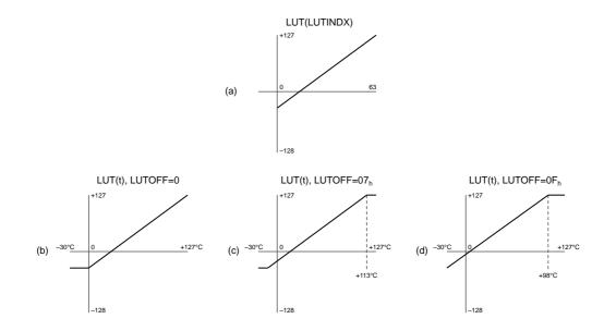
Figure 12. Examples of LUTOFF Operation
