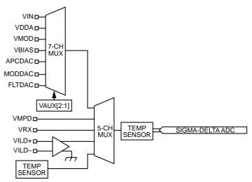
Figure 2. Analog-to-Digital Converter Block Diagram
