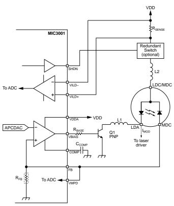
Figure 27. Example APC Circuit for Common Anode TOSA
