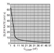
Figure 28. Slew Rate vs. C<sub>COMP</sub> Value
