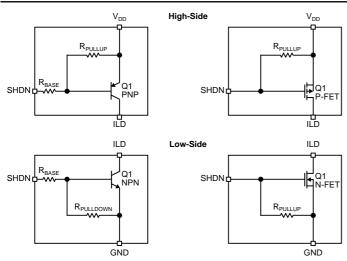
Figure 34. Redundant Switch Circuits
