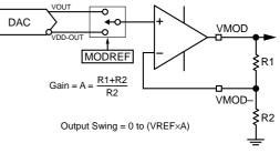
Figure 7. V<sub>MOD</sub> Configured as Voltage Output with Gain
