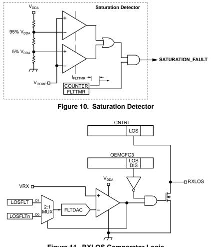
Figure 11. RXLOS Comparator Logic
