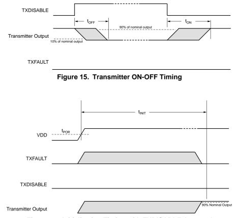
Figure 16. Initialization Timing with TXDISABLE Asserted
