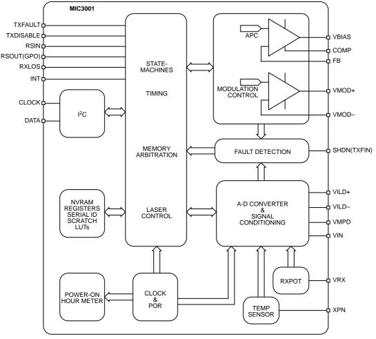
Figure 1. MIC3001 Block Diagram
