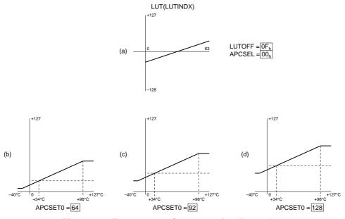
Figure 13. Temperature Compensation Examples
