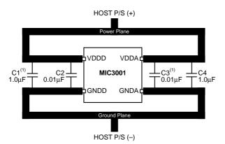
Figure 37. Power Supply Routing and Bypassing
