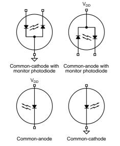
Figure 6. Transmitter Configurations Supported by MIC3001
