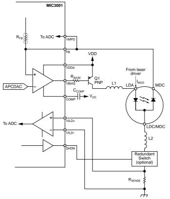
Figure 26. Example APC Circuit for Common-Cathode TOSA
