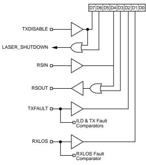
Figure 14. Control and Status I/O Logic
