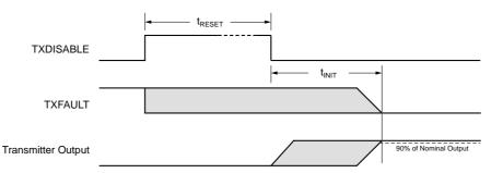
Figure 20. Successfully Clearing a Fault Condition
