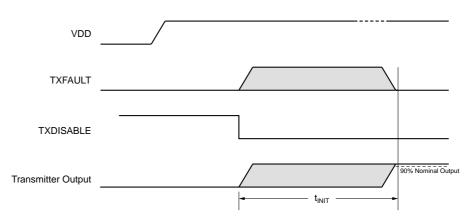
Figure 17. Initialization Timing, TXDISABLE Not Asserted
