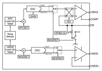
Figure 4. MIC3001 APC and Modulation Control Block Diagram
