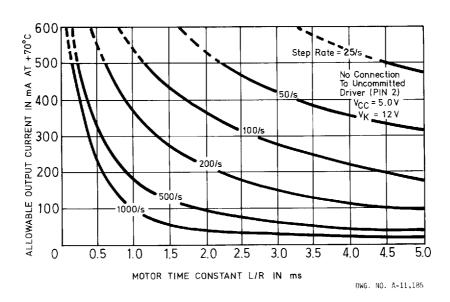
Notes: 1. Values shown take into account static d-c losses ( $V_{SAT}I_{OUT}$  and  $V_{CC}I_{CC}$ ) as well as switching losses induced by inductive flyback through the clamp diodes at  $V_K = 12$  V. Maximum package power dissipation is assumed to be 1.33 W at  $+70^{\circ}$ C. Higher package power dissipation may be obtained at lower operating temperatures.
