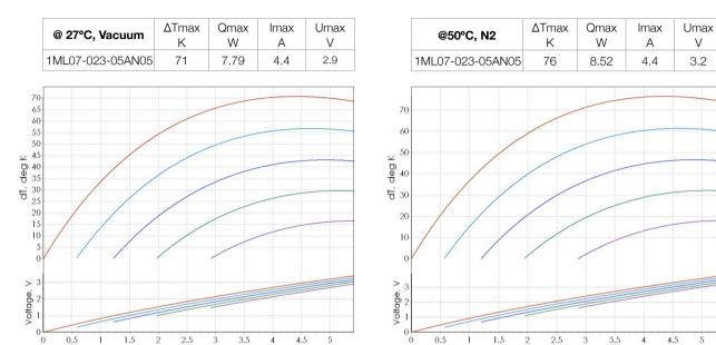
**Note**: Performance data is specified for optimal optimal conditions (TEC hot side is stabilized at ambient temperature). Heatsink thermal resistance is not included into estimations. Use TECCad Software for estimations under different conditions.
