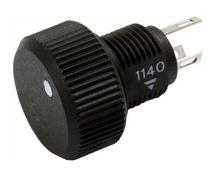
The P16 is a revolutionary concept in panel mounted potentiometers. This unique design consists of a knob driving and incorporating a cermet potentiometer. Only the mounting hardware and terminals are situated on the back side of the panel reducing to a minimum the required clearance.
