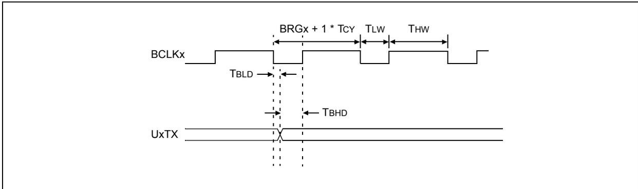
**FIGURE 28-9: START BIT EDGE DETECTION**
