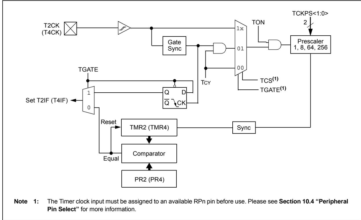
**FIGURE 12-3: TIMER3 AND TIMER5 (16-BIT ASYNCHRONOUS) BLOCK DIAGRAM**
