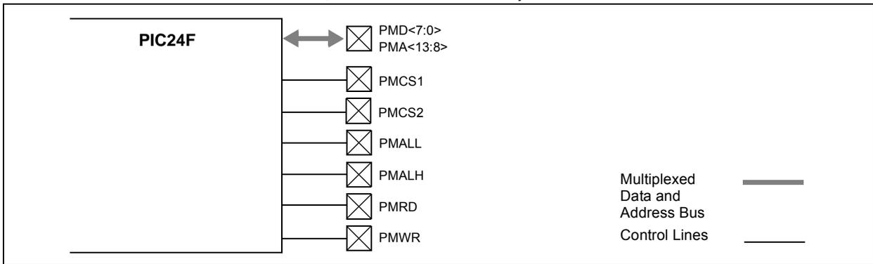
**FIGURE 18-7: EXAMPLE OF A MULTIPLEXED ADDRESSING APPLICATION**
