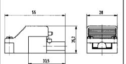
single screw connector strain relief for one round cable diameter 6.5-8.3 mm
