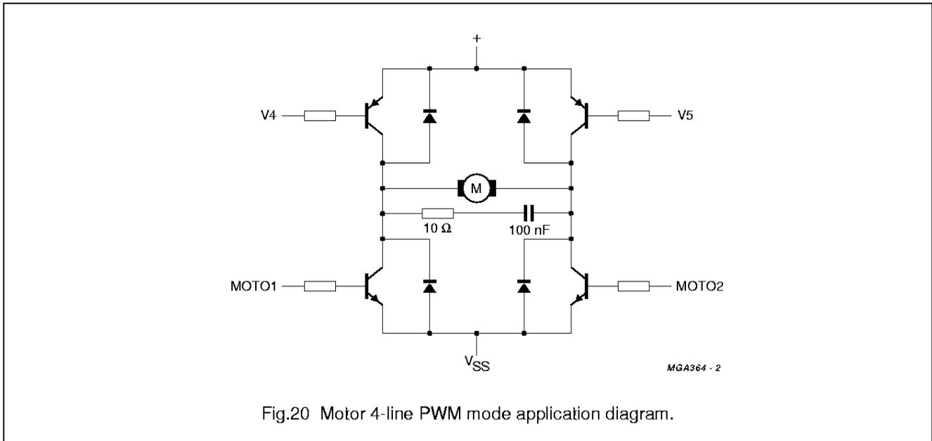
Fig.20 Motor 4-line PWM mode application diagram.
