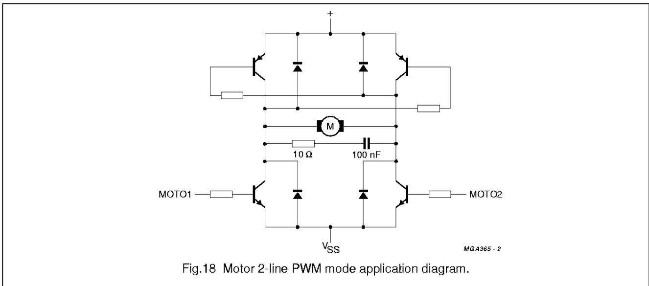
Fig.18 Motor 2-line PWM mode application diagram.
