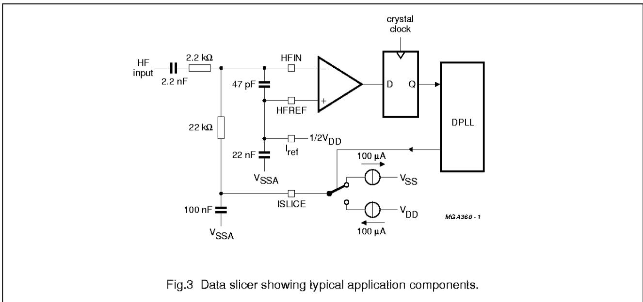
Fig.3 Data slicer showing typical application components.
