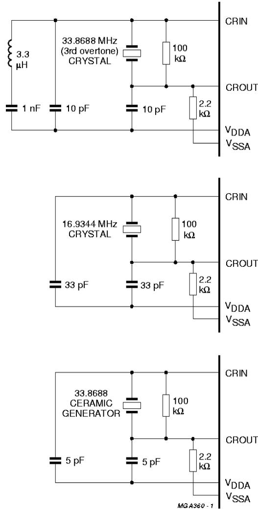
Fig.26 Application circuits for crystal oscillator.
