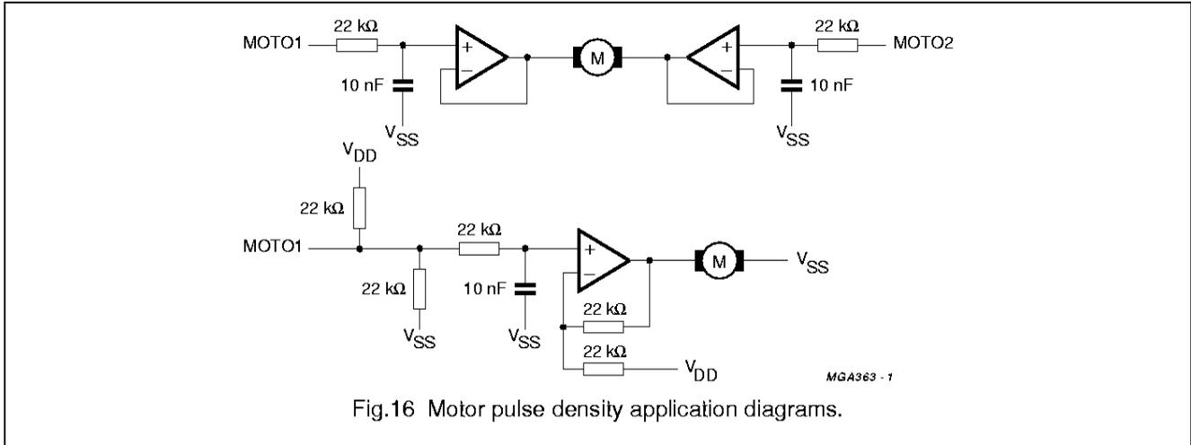
Fig.16 Motor pulse density application diagrams.
