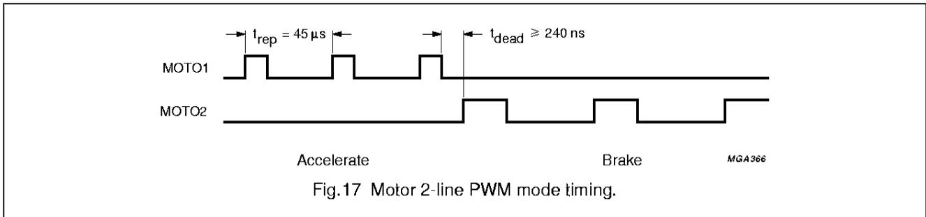
Fig.17 Motor 2-line PWM mode timing.
