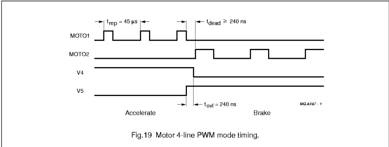
Fig.19 Motor 4-line PWM mode timing.
