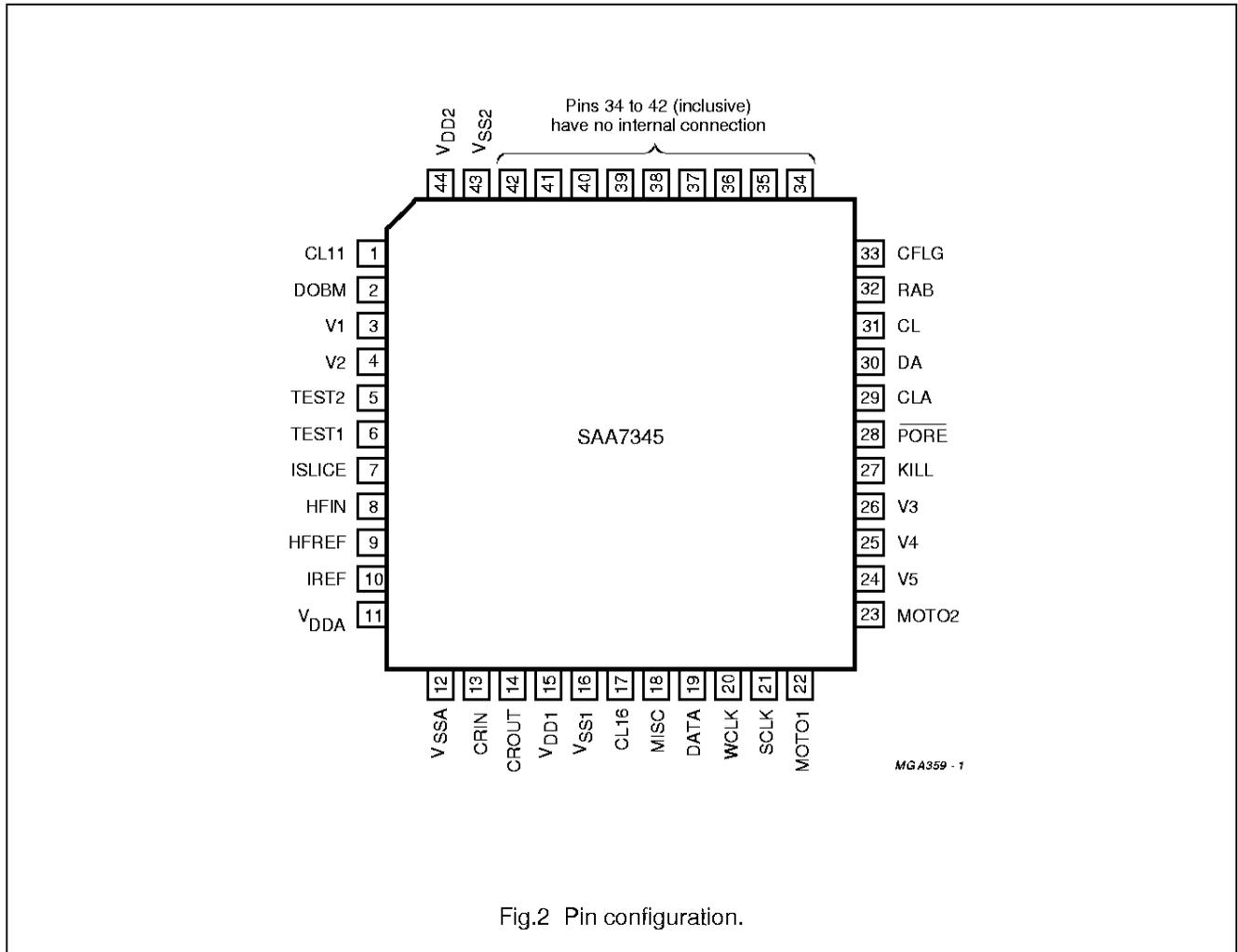
Fig.2 Pin configuration.
