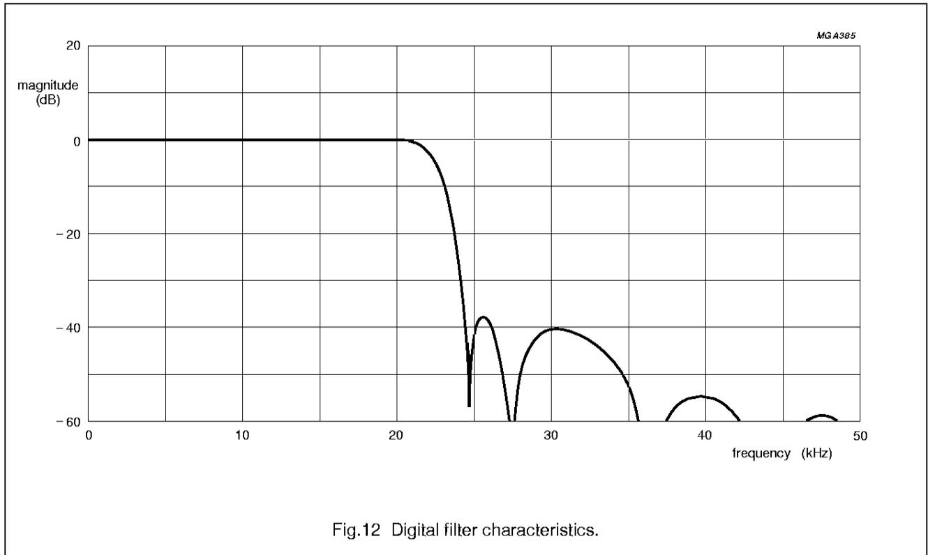
Fig.12 Digital filter characteristics.
