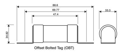
The range of Joint Service Fuse Links was originally developted for the Admiralty, but is now classified under the N.A.T.O. Reference system - Ref. Number 5920.99 The fuse links have been type approved and include short circuit tests to BS88, at 440 volts 33kA.
