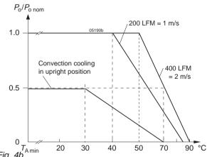
Output power versus temperature  $T_A$  at  $V_{inom}$  (CPD/CPA250)
