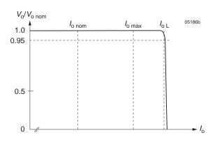
Fig. 3 Typical output characteristic V<sub>o</sub> versus I<sub>o</sub>
