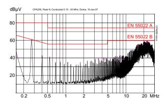
Fig. 13b Typical disturbance voltage (peak) at the line input according to EN 55022, measured at  $V_{\rm i\ nom}$  and  $I_{\rm o\ nom}$  (CPA250-4530).
