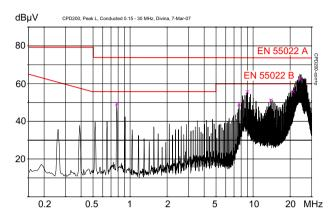
Fig. 13a Typical disturbance voltage (peak) at the negative input according to EN 55022, measured at  $V_{i \text{ nom}}$  and  $I_{o \text{ nom}}$  (CPD200-4530).
