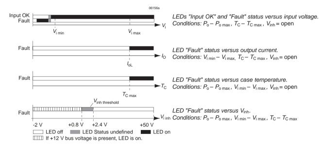
Fig. 12 Display status of LEDs
