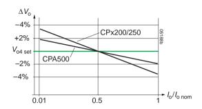
Fig. 11 Output voltage  $V_{04}$  versus output current  $I_{04}$ .
