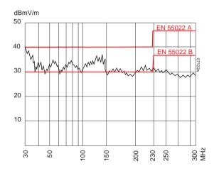
Fig. 14 Typical radiated electromagnetic field strength (quasi peak) according to EN 55022, normalised to a distance of 10 m, measured at  $V_{i \text{ nom}}$  and  $I_{o \text{ nom}}$ .
