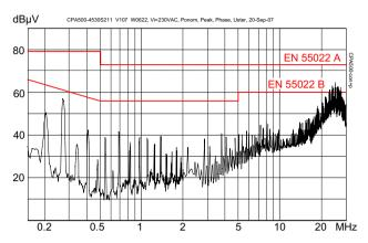
Fig. 13c Typical disturbance voltage (peak) at the line input according to EN 55022, measured at  $V_{\rm i \ nom}$  and  $I_{\rm o \ nom}$  (CPA500-4530).
