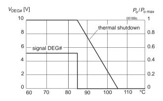
Fig. 9 Degrade signal  $V_{\text{DEG\#}}$  versus case temperature  $T_{\text{C}}$
