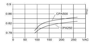
Fig. 2 CPA Series: Efficiency versus input voltage
