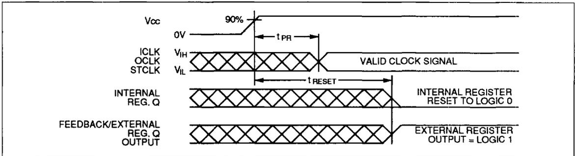
Circuitry within the GAL6001 provides a reset signal to all registers during power-up. All internal registers will have their Q outputs set low after a specified time ( $t_{RESET}$ , 45 $\mu$ s). As a result, the state on the registered output pins (if they are enabled) will always be high on power-up, regardless of the programmed polarity of the output pins. This feature can greatly simplify state machine design by providing a known state on power-up.
