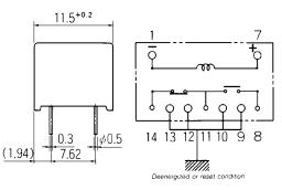
PC board mounting hole layout (Bottom view)
