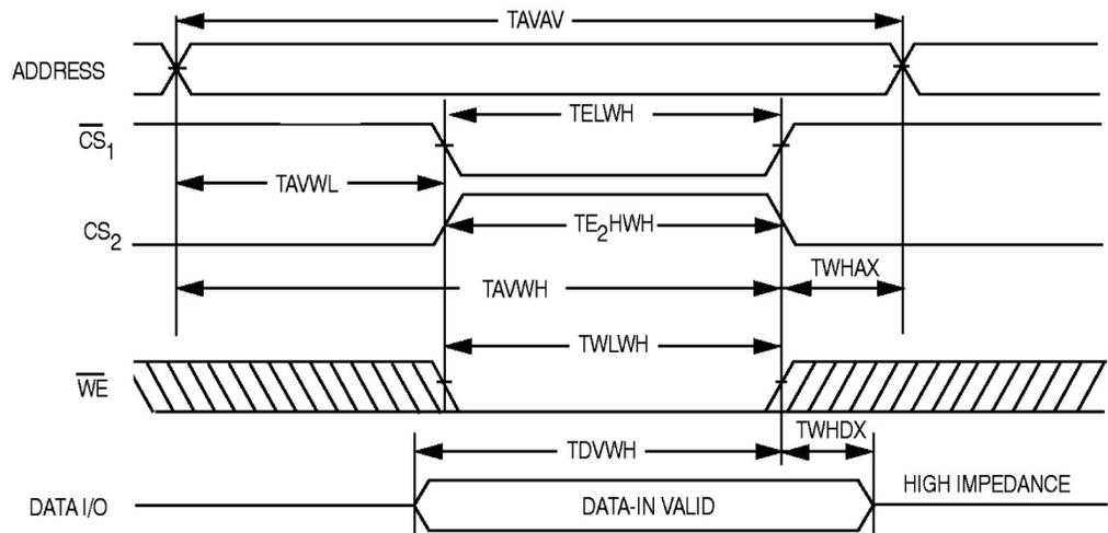
Note: The internal write time of the memory is defined by the overlap of  $\overline{CS1}$  Low and  $\overline{CS2}$  High and  $\overline{WE}$  Low. Both signals must be activated to initiate a write and either signal can terminate a write by going inactivated. The data input setup and hold timing should be referenced to the active edge of the signal that terminates the write. Data out is high impedance if  $\overline{OE} = V_{IH}$ .
