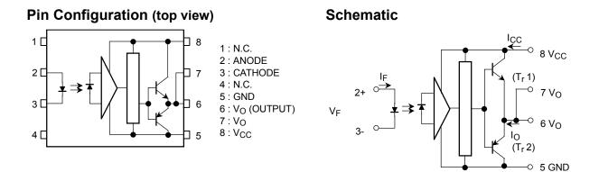
(Note 2) A 0.1  $\mu F$  bypass capcitor must be connected between pin 8 and 5.
