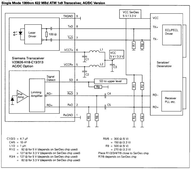
Values of R1/2/3/4 may vary as long as proper 50  $\Omega$  termination to V<sub>EE</sub> or 100  $\Omega$  differential is provided. The power supply filtering is required for good EMI performance. Use short tracks from the inductor L1/L2 to the module V<sub>CC</sub>Rx/V<sub>CC</sub>Tx.
