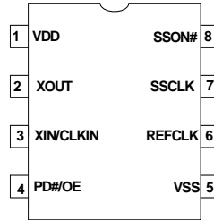
Figure 1. CY25100 8-Pin SOIC/TSSOP
