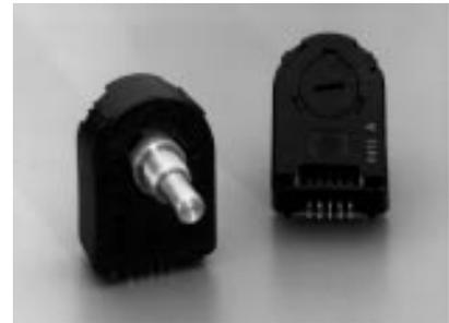
life, and increased reliability. The unit outputs two digital waveforms which are 90 degrees out of phase to provide position and direction information. The HEDS-5740 Series provides a third Index Channel.
