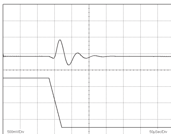
Figure 6: Typical Transient Response 75-50% Step Load Change (1A/µsec), Top (Vout) Bottom (Iout)
