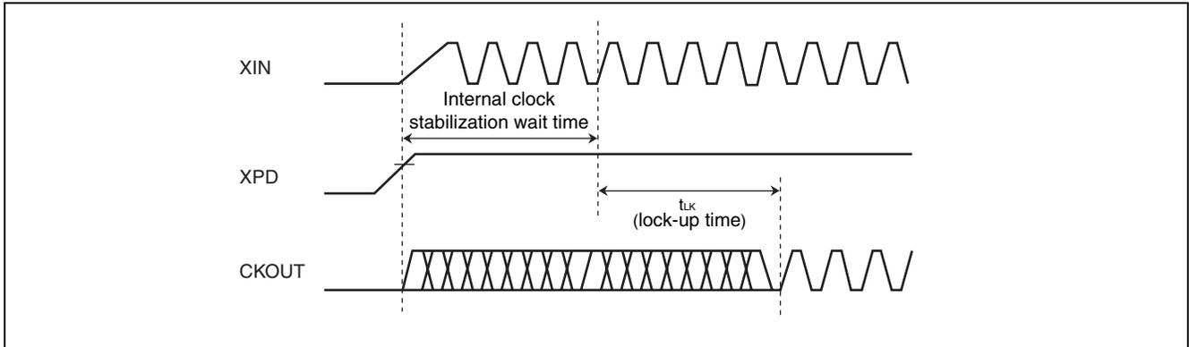
When the power down is controlled by XPD pin, the desired clock is obtained after the pin is set to H level until the maximum lock-up time  $t_{LK}$  is elapsed.
