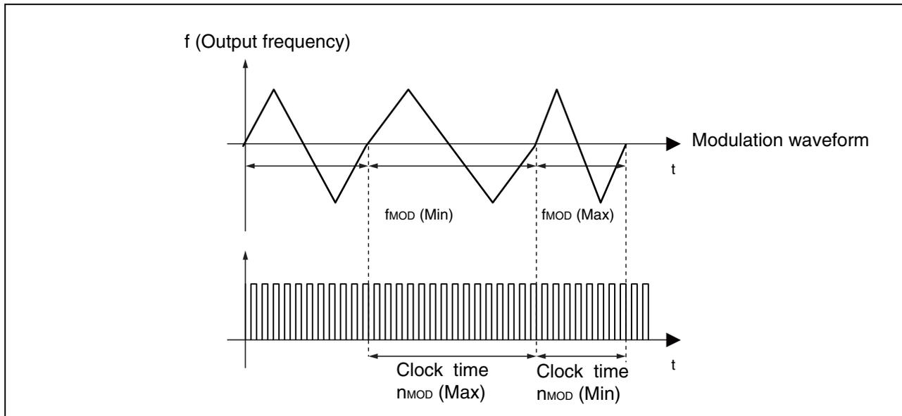
MB88151A contains the modulation period to realize the efficient EMI reduction.
