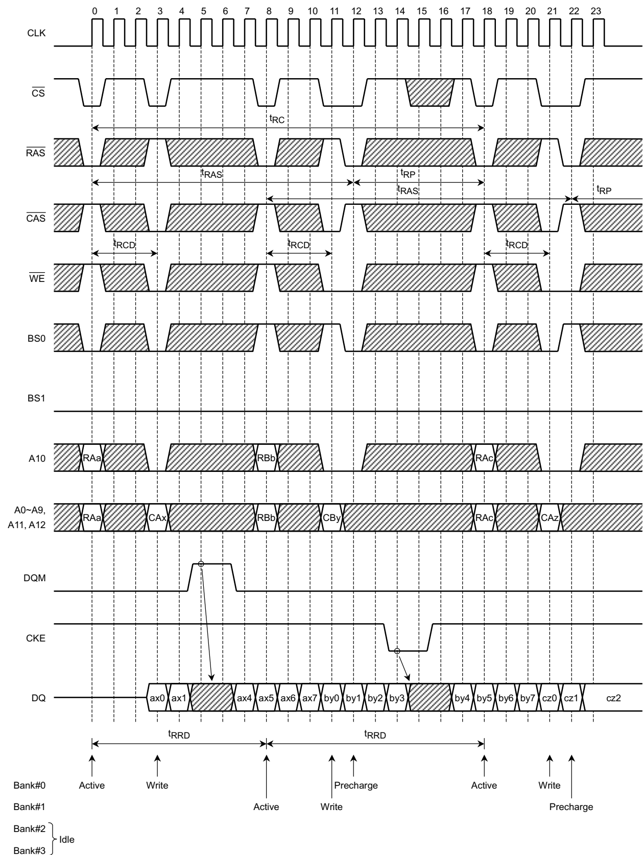
Figure 5. Interleaved Bank Write (Burst Length = 8)
