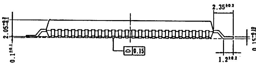
ES 80-pin Ceramic Flat Package (for reference) (unit: mm)
