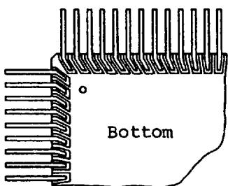
1. Note that the metal cap that is connected to pin 33 becomes the positive power supply level.
