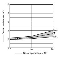
7-(2). Electrical life test (Lamp load)
